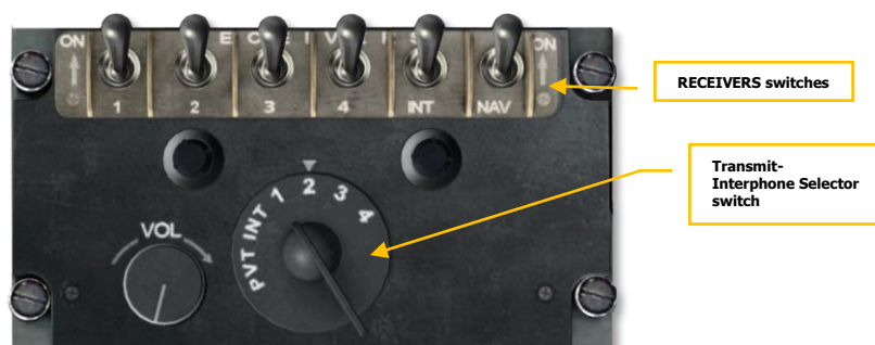
Figure 7.1.1. C-1611/AIC Signal Distribution Panel
