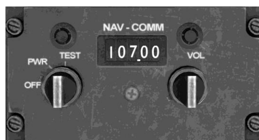
Figure 7.2.1 Navigation Control Panel AN/ARN-82
