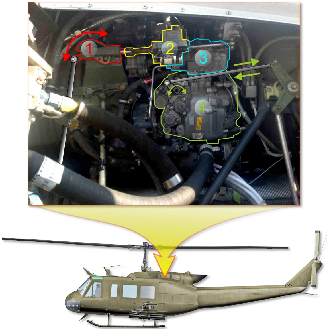
Figure 2.8. Engine Mounted Components.
