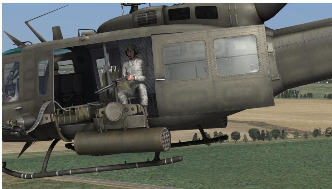
Figure 8.1. The flexible 7.62 millimeter machine guns M60D on the right board
