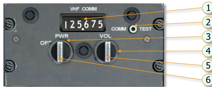
Figure 7.1.3 VHF Control Panel C-7197/ARC-134
